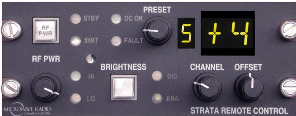
STRATA TRANSMIT REMOTE CONTROL PANEL AND DISPLAY: (ACTUAL SIZE)
