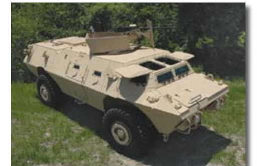
The Iraqi Armored Personnel Carrier ASV variant is configured for transport of a crew of 10 (driver, commander, and eight passengers).
