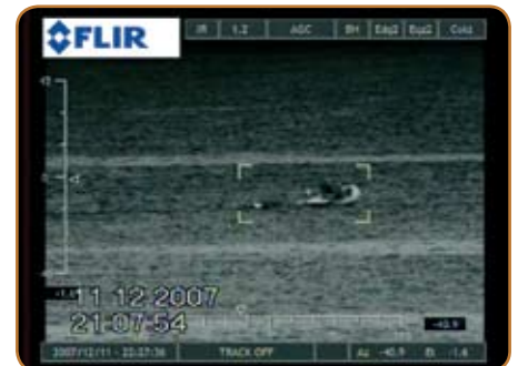
Equipped with a video tracker, the Multi-Sensor systems can follow an object as long as it can be seen.
